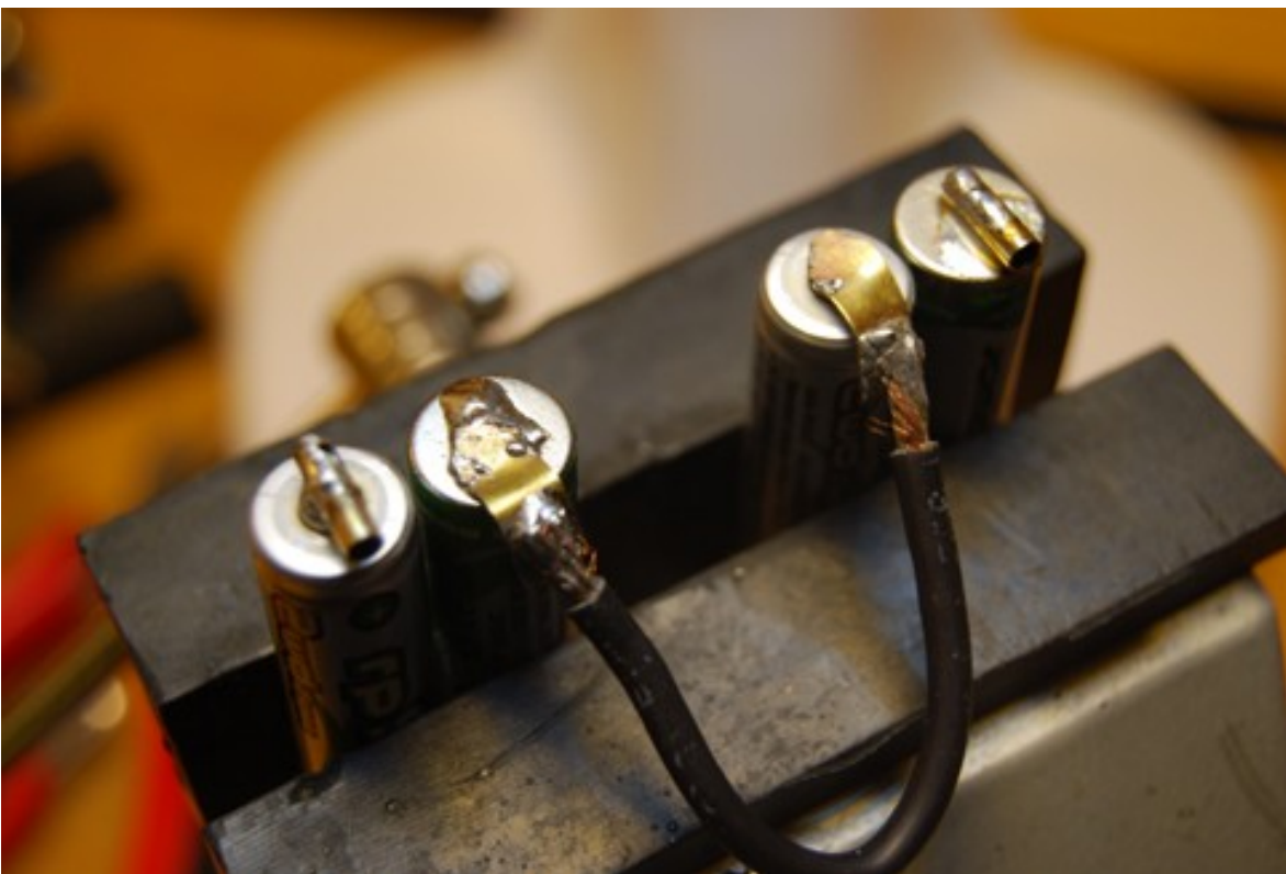
Fig 9 Mounted connection wire.
